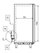
Electrical inlet (power) RO Refrigerant Outlet
